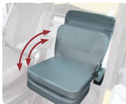
The full size trainer seat has a foldable cushion and back rest for easy cab entry and access to the air conditioner filter and glove compartment
