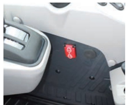
Secondary engine shutdown switch
