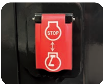
Secondary engine shutdown switch
