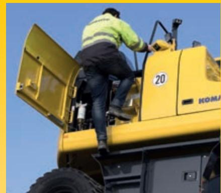
*Handrails and anti-slip plates*
